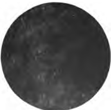
Fig. 25. Temper drawn at 400 Degrees C.; Osmondite Structure
